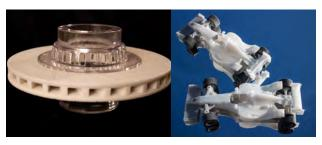
Multi-material composite parts, built in one part/one time
