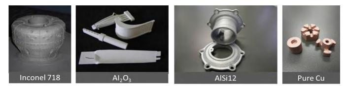
Parts can be printed in a variety of ferrous and non-ferrous metals, and ceramics.
