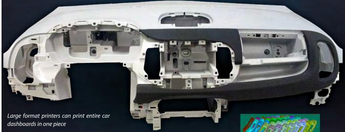
In functional testing, it is specifically important to build parts in one piece. If your part size exceeds your build volume, there still is the option to join parts. Be aware however that joining affects part functionality. Mechanical testing on a joined part will not accurately reflect the performance of a part that will later be produced in one piece.
