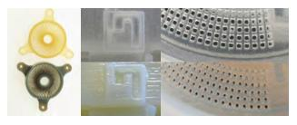
Compare razor sharp edges and corners definition, round circles, minimum feature size, sidewall quality and surface smoothness
