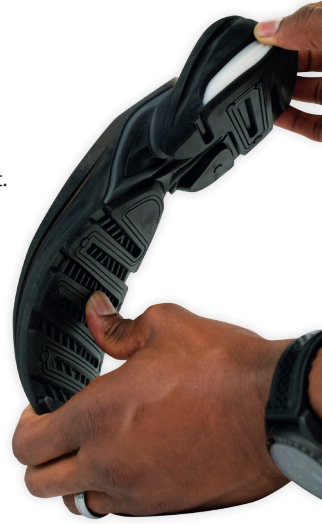
Shoe sole printed at one time in a combination of flexible black elastomer and rigid white plastic
